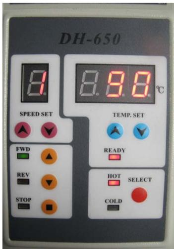
For sensitive media like PE film, set the temperature to approx. 90° C (195° F) and a slow speed (1-2 on the DH-650 model). For thicker media with rough surfaces like cardboard or heat-resisting materials like sheet-metal, a higher temperature of up to 170° C (340° F) is recommended. In general, always use the highest temperature, depending on the substrate. Make sure that the pressure rollers are in the 'close' position.
