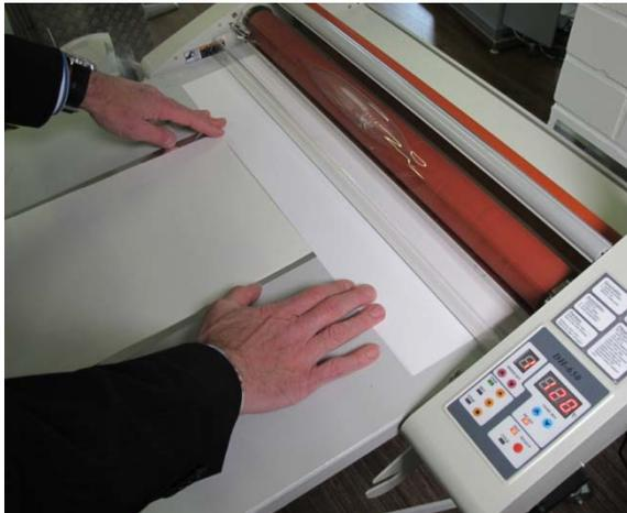
Hold the transfer film and the substrate together and push them onto the pressure rollers until the roller have caught and transport the material. Do not use the full width of the laminator; otherwise the material gets damaged if not fed in straight.
